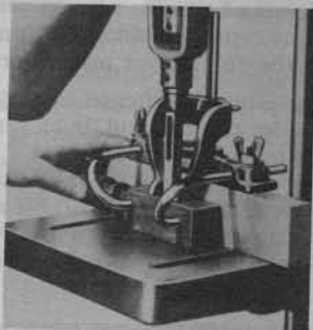
Mortising is one of many useful operations . . . a necessity in making mortise and tenon joints.
