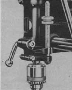
Quill lock and adjustable stop permit precision adjustment for repeating.
