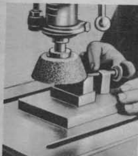
Drill Press provides fast, accurate method of surface grinding in the home workshop.
