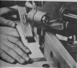
Many beautiful shaped edges can be made on the drill press—using the shaper attachment.
